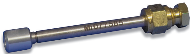
Standard sorbent tube fitted with a diffusion cap at the sampling (grooved) end
